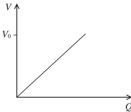
At a potential difference  $V_0$  a small charge  $\Delta Q$  is added to the capacitor. This results in a small increase in potential difference  $\Delta V$  across the capacitor.
