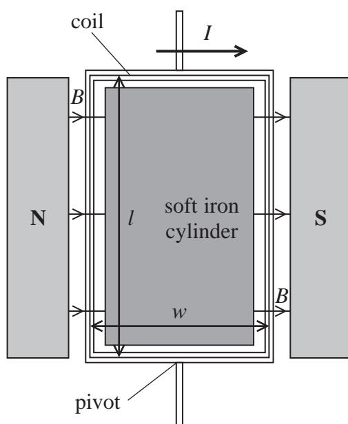
The fixed soft iron cylinder and magnets produce a uniform magnetic field of magnetic flux density  $B$ . The coil is able to rotate within this magnetic field. The coil has width  $w$  and length  $l$ . There is a current  $I$  in the coil in the direction shown in the side view diagram.
